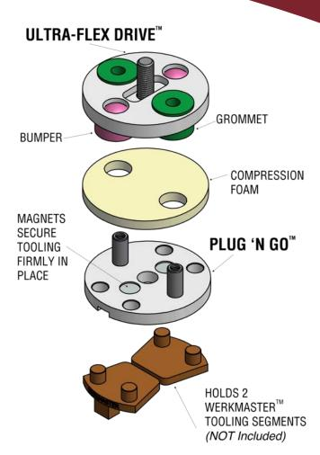
Just PLUG 'N GO. When it comes to all WerkMaster machines, putting on and removing your tooling is a breeze. Strong earth magnets and clip-in tooling save time on any job
